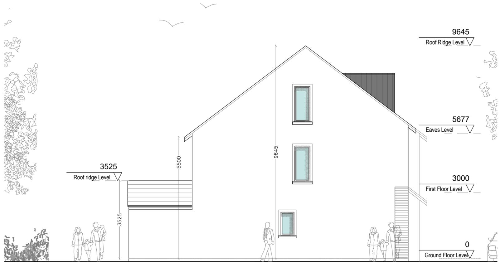
Proposed Side Elevation \* FINISHED FLOOR LEVELS - REFER TO SITE LAYOUT PLAN
