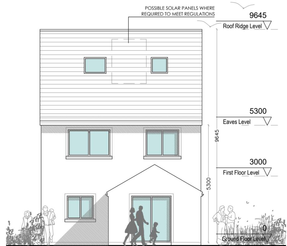
Proposed Rear Elevation \* FINISHED FLOOR LEVELS - REFER TO SITE LAYOUT PLAN
