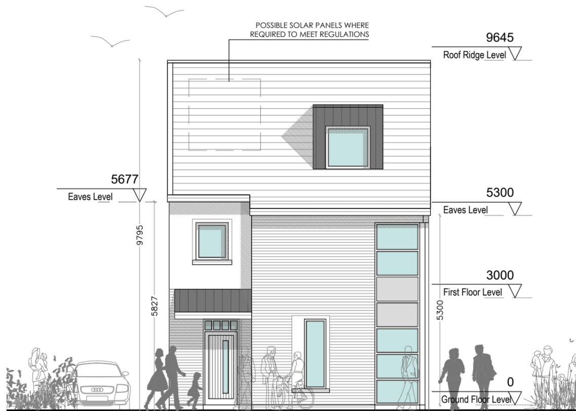
Proposed Front Elevation \* FINISHED FLOOR LEVELS - REFER TO SITE LAYOUT PLAN
