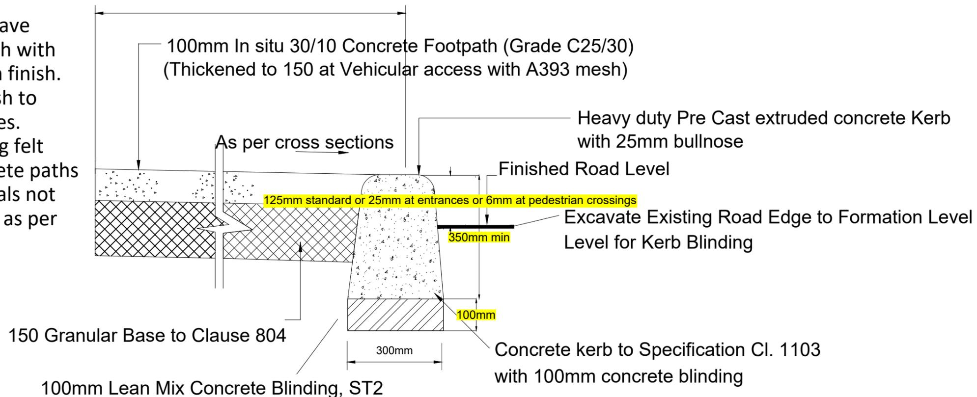
**Pre-Cast Concrete Kerb Detail**
