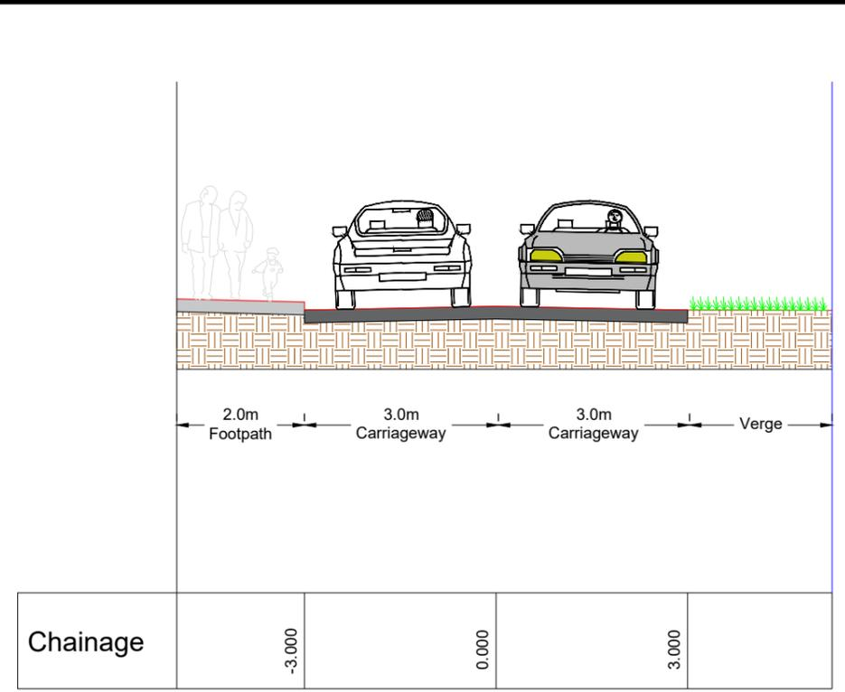
Typical Cross Section - Estate Road (Footpath on One Sides)
