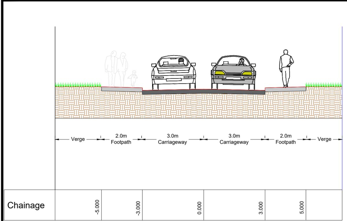
Typical Cross Section - Estate Road (Footpath on Both Sides)
