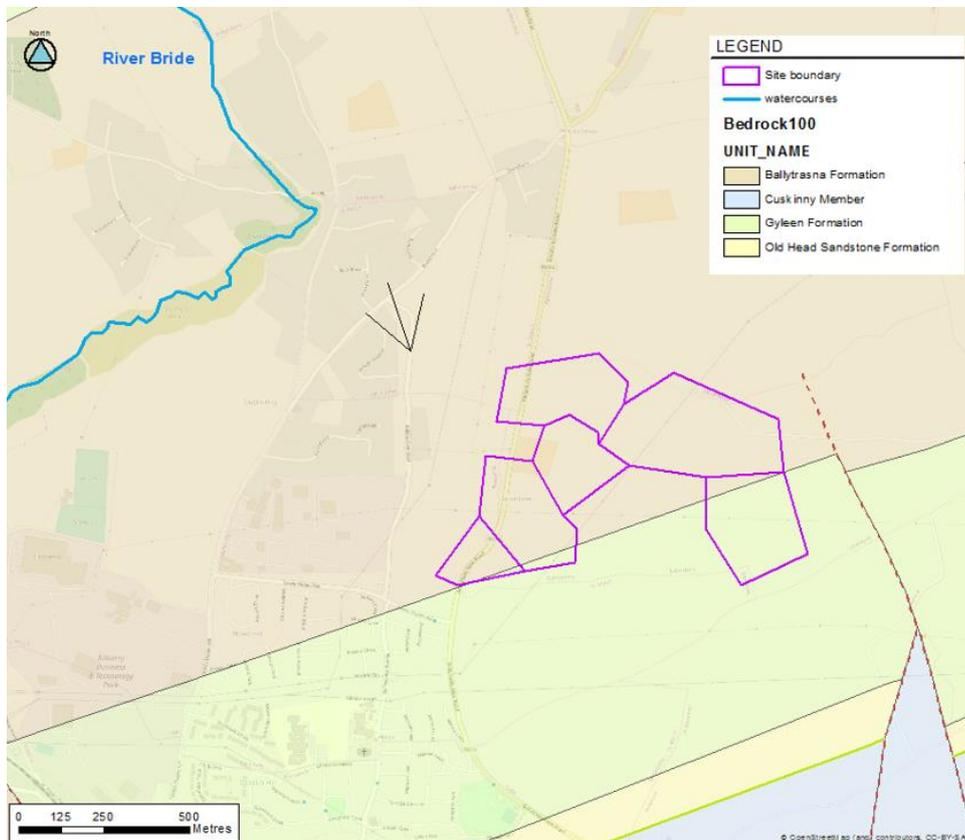
The bedrock is largely covered by till derived from Devonian sandstones. In the south east of the site there are gravels derived from Devonian sandstones. In the surrounding region, there are localised areas of bedrock exposed at the ground surface and Made Ground (Urban) areas lie in Cork to the south. Superficial deposits are shown in Figure 2-3.
