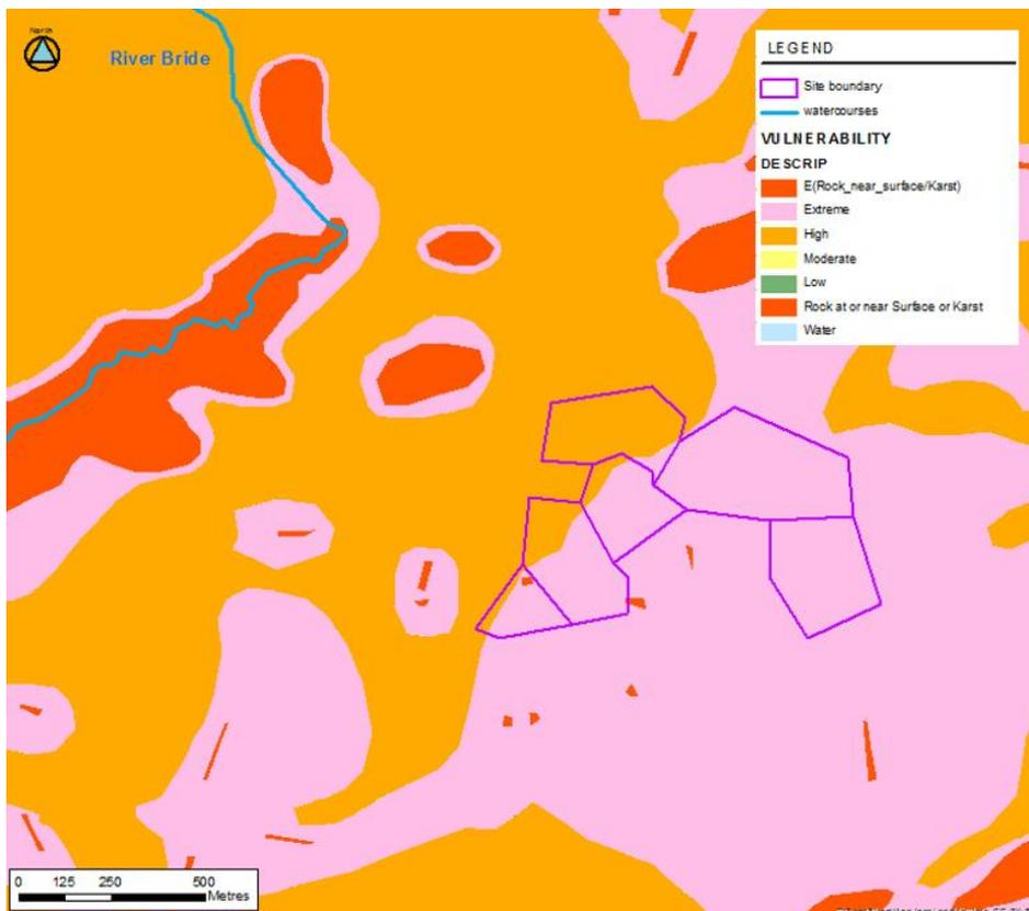
The regional groundwater flow direction is likely to echo that of topography and catchment drainage and, in the absence of more detailed groundwater level data, would be expected to be flowing south west to the River Bride. Locally to the site, groundwater is likely to flow from the higher ground in the east towards the depression west of the site.
