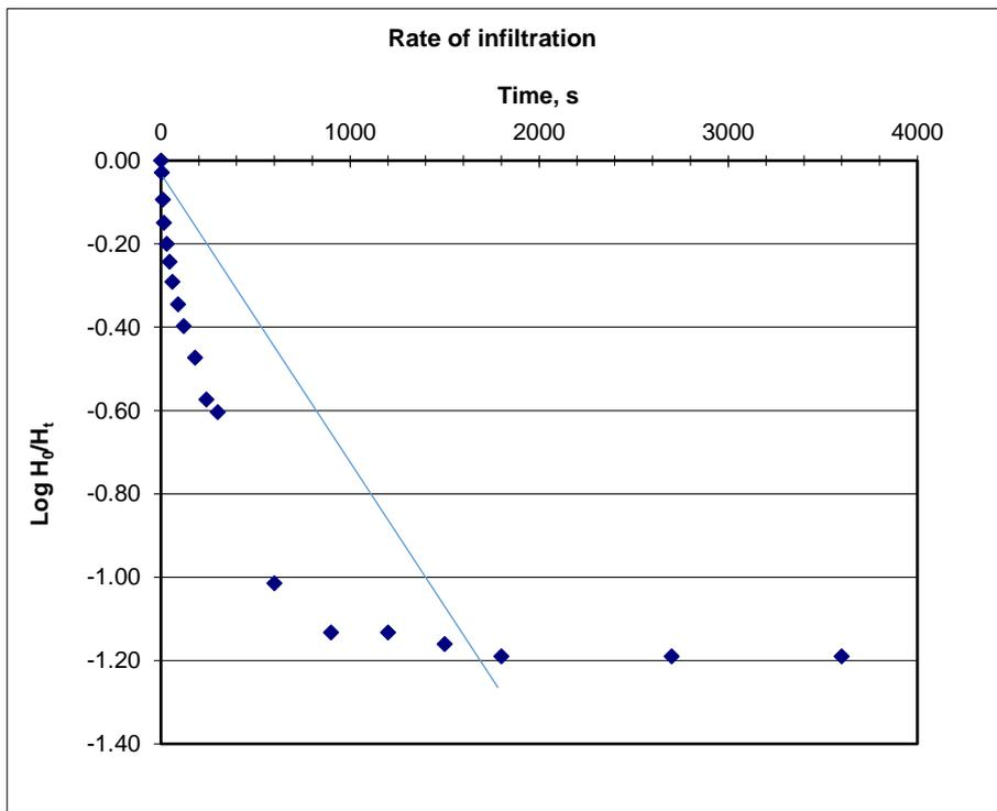
**P19012 Falling head permeability test**
