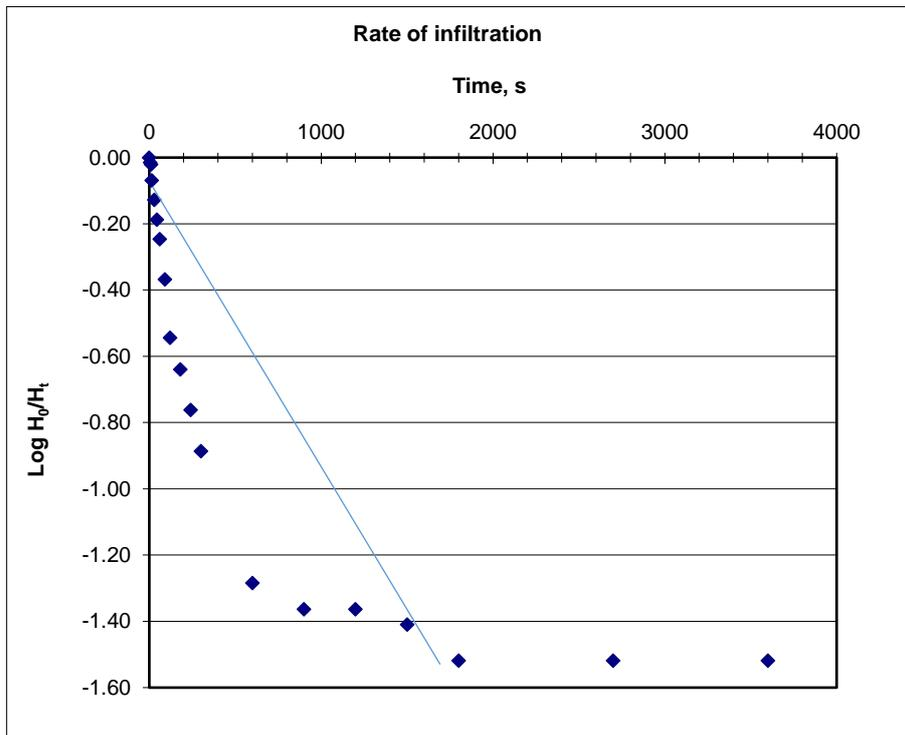
**P19012 Falling head permeability test**
