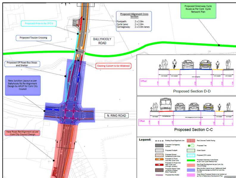
**Fig 7.1: Junction 1, Proposed Upgrade Works**
