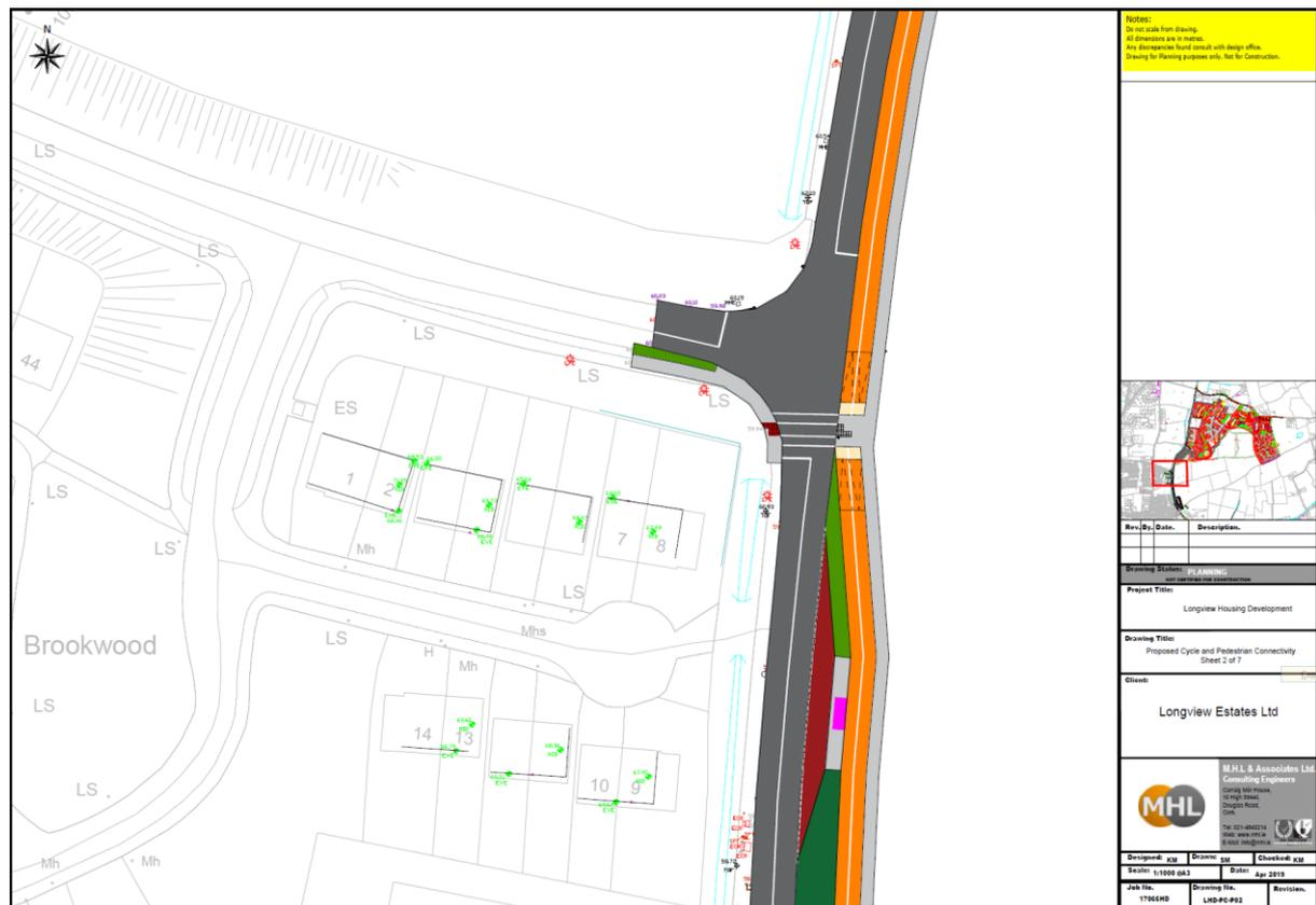
**Fig 12.1: Proposed New Bus Stop on the R614 and two-way cycle lanes**
